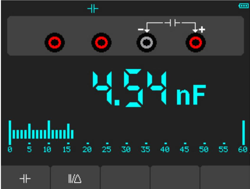
Figure 4-5 Capacitance Measurement
