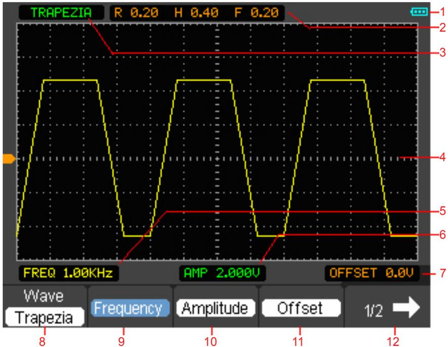
Figure 5-1 Waveform Generator Display Screen
