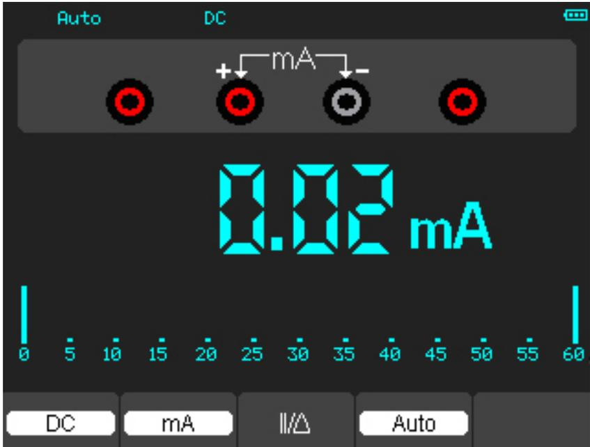
Figure 4-8 DC current Measurement for 600 mA
