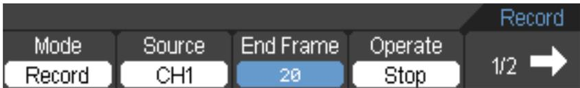
Figure 2-48 The Recorder menu (Record Mode)
