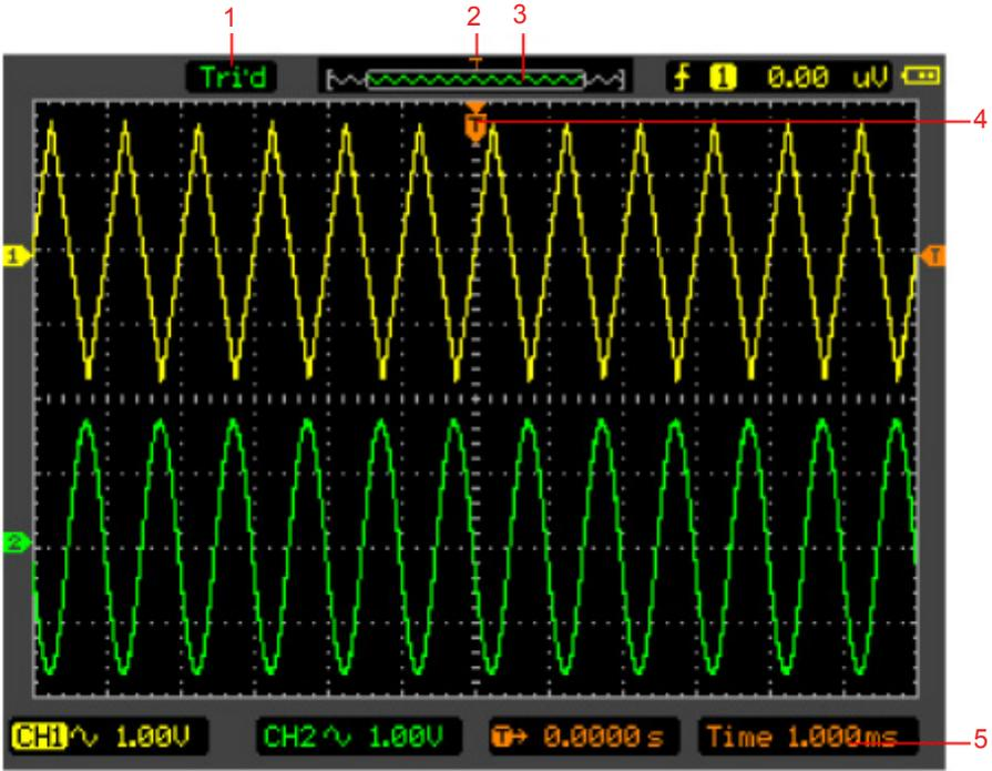
Figure 2-23 The horizontal/Time base marks
