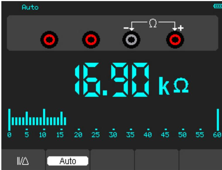
Figure 4-2 Resistance Measurement
