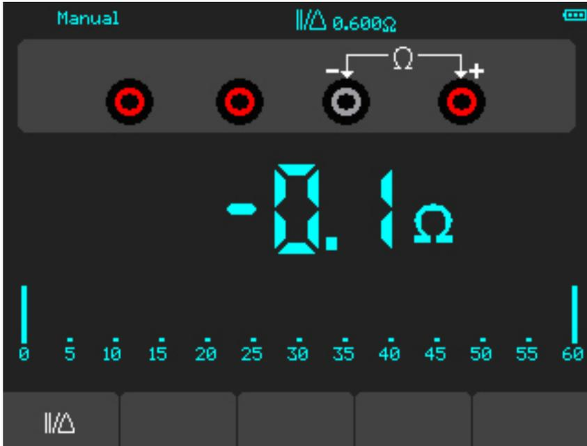
Figure 4-12 Relative Measurement
