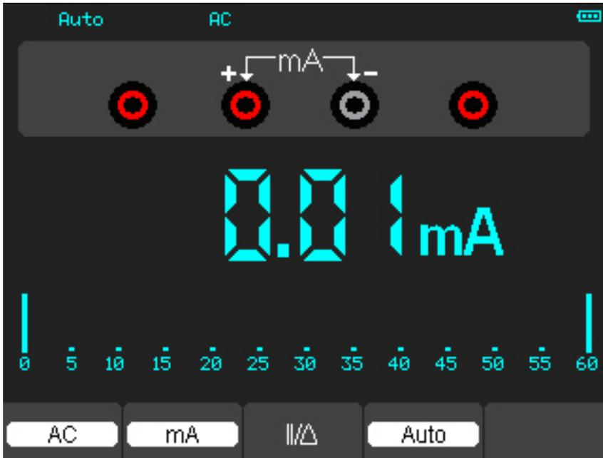
Figure 4-10 AC Current Measurement for 600 mA
