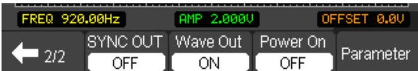
Figure 5-11 The Waveform Generator menu
