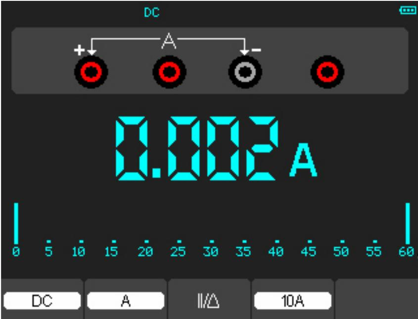
Figure 4-9 DC Current Measurement for 10A
